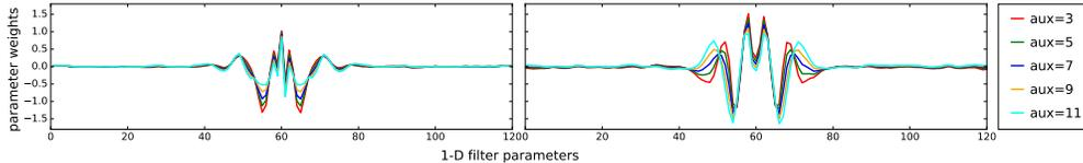
**Figure 8:** Two examples of filter manifolds for image deconvolution. The y-axis is the filter weight, and x-axis is location. The auxiliary input is the disk kernel radius. Both the amplitude and the frequency can be adapted.
