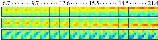
**Figure 6:** Examples of learned filter manifolds for the 2nd convolutional layer. Each row shows one filter as a function of the auxiliary input (perspective weight), shown at the top. Both the amplitude and patterns change, which shows the adaptability of the ACNN.
