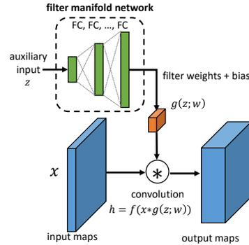
**Figure 2:** The adaptive convolutional layer with filter manifold network (FMN). The FMN uses the auxiliary input to generate the filter weights, which are then convolved with the input maps.
