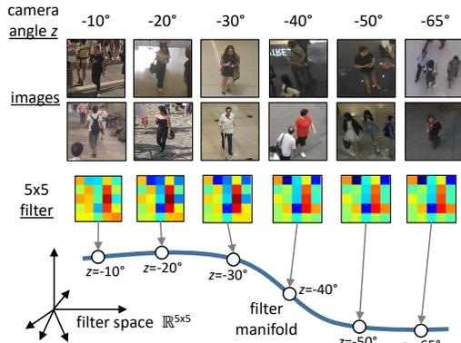
**Figure 1:** (top) changes in people’s appearance due to camera angle, and the corresponding changes in a convolution filter; (bottom) the filter manifold as a function of the camera angle. Best viewed in color.
