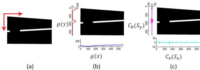
**Figure 4: Computing splitting line.** (a) current block to be split. (b) accumulated pixel values along horizontal and vertical directions. (c) the cost functions of placing a splitting line along horizontal and vertical directions.
