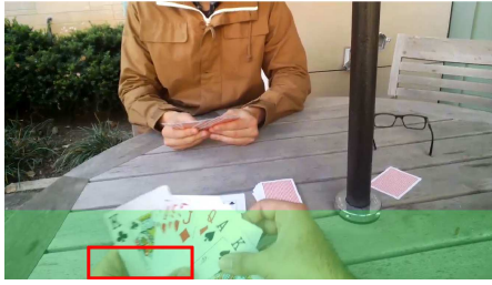
Fig. 2. ZOOM takes as input one fourth of the image (green), and the bounding boxes that entirely fall into that area (red box) as ground truth.
