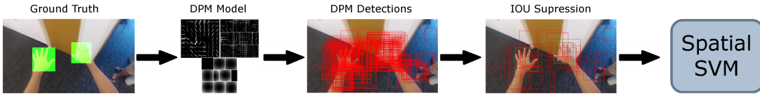
Fig. 2. Training pipeline of our proposal generation method. We use the bounding box ground truth to train the DPM and find the different appearances. To train the Spatial SVM we use the DPM to detect the hands on the training dataset and suppress the detections using IOU suppression. As positives we use the detections whose intersection over union with the ground truth is over 0.5, every other detection is taken as negative.
